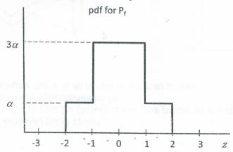
Note: it is NOT needed to solve the problem, but the variable  $z = \left(log(\overline{N_f}) - log(N_f)\right)/\sigma_N$  where  $\overline{N_f}$  is the average fatigue life and  $\sigma_N$  is the standard deviation in  $(N_f)$ .
