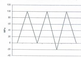
A component constructed from this material is loaded with the above nominal stress sequence. Assume  $K_t = 1.5$ .
