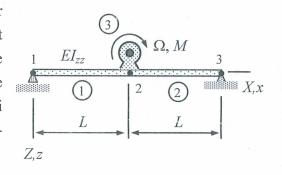
4. The Bernoulli beam shown is subjected to force F at node 2, when t < 0. At t = 0, the force is suddenly removed and the beam starts to vibrate. Derive the ordinary differential equation and initial conditions giving the displacement  $u_{Z2} = a$  as function of time  $(\theta_{Y2} = 0)$  for t > 0. The beam is thin so that the rotational part of the inertia term is negligible. The geometrical quantities of the cross-section are A,  $I_{zz}$  and the material constants E and  $\rho$ .
