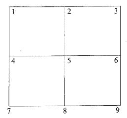
Hint: points 1, 2, 3, 4, 7 have a known constant temperature by construction. Exploit the symmetry of the system and use heat balance equations at points 5, 6, 8 and 9.
