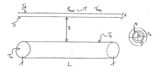
Assuming that the winter design temperature for the outside is  $T_{ext} = -15$ °C and steady-state heat transfer occurs, find the minimum depth z so that the external surface of the pipe (at  $D_2$ ) is at the freezing point. The heat loss at the ground level is  $q'' = 20W/m^2$  on an
