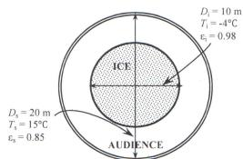
Assume that the ceiling is dome-shaped, with emissivity  $\varepsilon_c = 0.28$ , height H=10m and average temperature  $T_c = 7$ °C. The circular ice rink has diameter  $D_i = 10$ m,  $T_i = -4$ °C and  $\varepsilon_i = 0.98$ . The audience's sitting area, between the rink's edge and the dome's walls, corresponds to  $D_s = 20$ m,  $T_s = 15$ °C and  $\varepsilon_s = 0.85$ .
