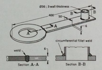
Note: All dimensions are in "mm" and manufacturing and quality inspection are performed indoors. The type of joint and bevel represented in the schematic drawing are only representative, i.e. any other more convenient should be adopted.
