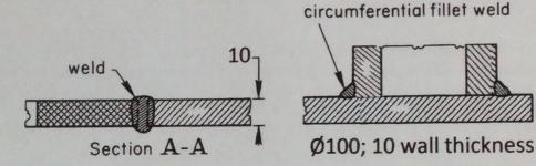
Note: All dimensions in "mm". Assume that the tube has circular section with infinite axial length and that the in-plane dimensions of the strip plate are infinite.
