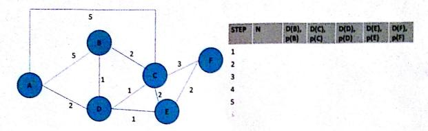
D(v) = cost of the path from the source to the destination v that has currently as of this iteration of the algorithm the least cost p(v)=previous node, neighbour of node v along the current least-cost path from the source to node v
