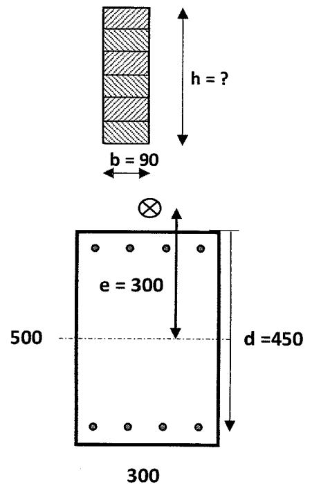
3. Cross-section of symmetrically reinforced concrete column is shown in the figure. Strength class of the concrete is C35 and the quality of steel is B500B. Loading is eccentric ( $e = 300$  mm) compressive load consisting of permanent  $N_g = 400$  kN and imposed load  $N_q = 700$  kN. Respective load factors are 1.15 and 1.5.
