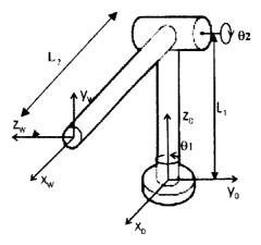
**4.** <u>Form the manipulator Jacobian matrix for the planar RR-manipulator shown in the figure below.</u> (11 points)
