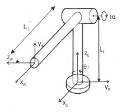
**4.** <u>Form the manipulator Jacobian matrix for the planar RR-manipulator shown in the figure below.</u> (11 points)
