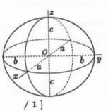
b) Derive the formula for intersecting a ray with the ellipsoid. The result is a quadratic equation in t with coefficients A, B, C. Like always, we will substitute the equation of the ray to the implicit equation of the ellipsoid.
