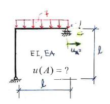
1X: [Extra, 1p] - Strain energy of a frame: write mathematically the expression of strain energy of a linear elastic frame accounting for bending, stretching and shearing a) in terms of internal forces [0.5 p] and b) in terms of corresponding generalized deformations [0.5 p]. (No need to account for  $2^{nd}$  order effects). /extra means that you can freely choose not to answer without losing points. However, right answer will count/
