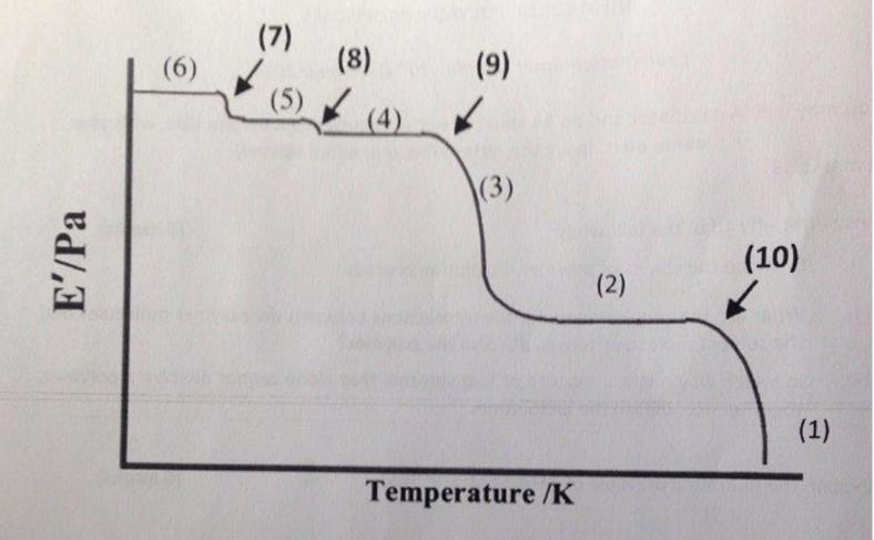
Figure 1. Idealized DMA curve for partially crystalline polymer
