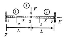
2. Determine the horizontal and vertical displacements of node 2. Cross-sectional area of bar 1 is  $\sqrt{2}A$  and that of bar 2 is A. Young's modulus of the material is E.
