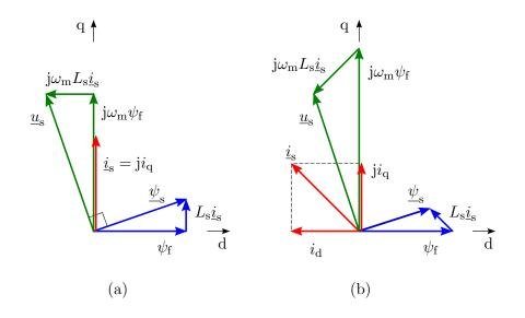
**Remark:** It can be noticed that the torque decreases more than inversely proportionally to the speed in the field-weakening region and the mechanical power decreases. In surface-mounted permanent-magnet machines, the d component of the current produces no torque; it only magnetises against the permanent magnets in order to decrease the stator flux magnitude.
