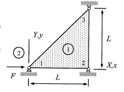
5. Determine the static displacements  $u_{Z2} = -u_{Z3}$  of nodes 2 and 3 due to the temperature increase  $\Delta \theta$  at nodes 2 and 3 (actually in the wall). The material constants are E and  $\alpha$ . The cross-sectional area of bar 1 and 3 is A and that of bar 2 is  $\sqrt{2}A$ . The initial temperature is  $\theta$ .
