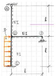
4. Use Slope-Deflection Method and derive the expression of the criticality condition to determine the critical buckling load for this continuous column [5p]. The bending rigidity of the column is twice the bending rigidity of the beam; El<sub>c</sub> = 2\* El<sub>b</sub>.
