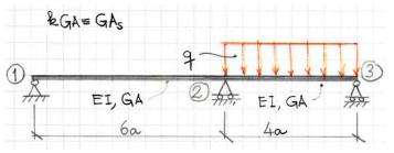
3. Use Slope-Deflection Method and determine the bending moment at the clamping support 1. [4 points] Determine and draw the bending moment diagram [1 point]
