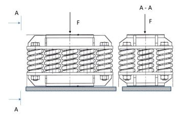
a) To describe the effect of bolt prestressing (F=0) on the spring unit, the unit can be divided into three main parts. Construct free-body diagrams to describe the effect of prestressing on the spring unit and its support by adding vertical reaction forces to the figures below. (4p)
