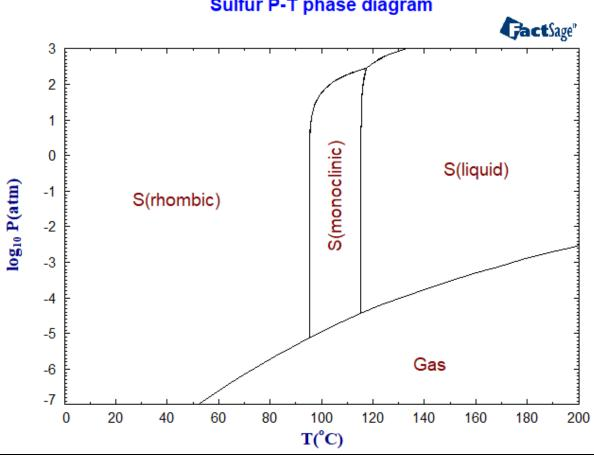
Sulfur P-T phase diagram
