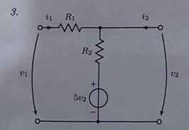
Determine the hybrid parameters of the circuit.
