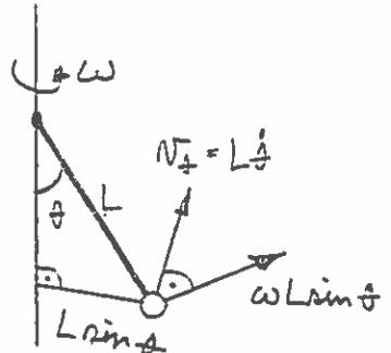
$$\begin{aligned} \frac{\partial L}{\partial \dot{\theta}} &= \frac{1}{2} m \omega^2 L^2 \cdot 2 \sin \dot{\theta} \cos \dot{\theta} - mg L \sin \dot{\theta} \\ &= mL \sin \dot{\theta} (\omega^2 L \cos \dot{\theta} - g) \end{aligned}$$
