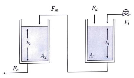
We are interested in controlling the level of water in the two tanks by manipulating the influent flow-rate  $F_i$  to the first tank. Moreover, we will assume that both  $h_1(t)$  and  $h_2(t)$  are measured quantities and that  $F_i(t)$ ,  $F_m(t)$ ,  $F_d(t)$ , and  $F_o(t)$  are measured, as well.
