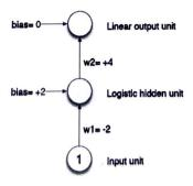
Figure 1: A small neural network with one hidden unit. The values for the weights and biases are given in the figure.
