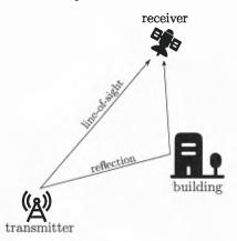
The transmitted signal arrives in two paths: a direct line-of-sight (LOS) path and slight reflection from a building nearby. The LOS path arrives at the receiver after N samples from the moment the signal gets transmitted. The reflected path travels a longer distance and arrives at the receiver 6 samples later. Additionally, the reflection absorbs 50% of the transmitted energy.
