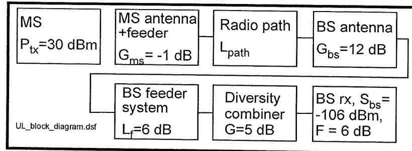
Determine using the COST231 Hata-model for average path loss calculation the maximum cell radius in a 420 MHz TETRA system used in a suburban environment, when the base station antenna height is 60 m, the mobile station antenna height is 1.6 m, and the shadow fading margin is 5 dB. The other link parameters are given in the figure above.
