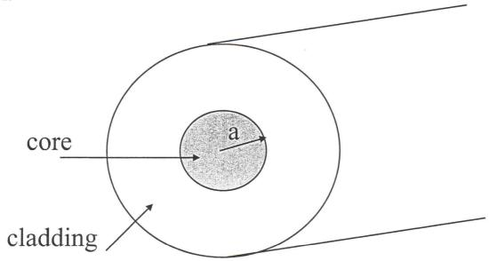
Consider light propagation in a step-index optical fiber (pictured above) with a core radius a, core refractive index  $n_{core}$  and cladding refractive index  $n_{clad}$ . The "characteristic equation" for a step index fiber can be written as:
