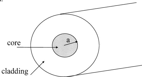
Consider light propagation in a step-index optical fiber (pictured above) with a core radius a, core refractive index  $n_{core}$  and cladding refractive index  $n_{clad}$ . The "characteristic equation" for a step index fiber can be written as:
