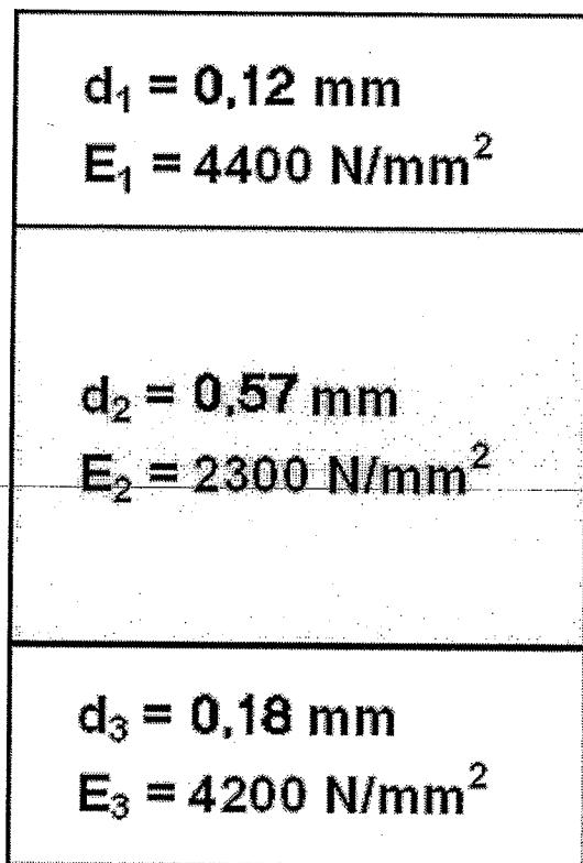
Figure 1. Structure of a 3-layer board (question 5)
