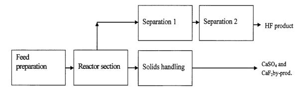
The block flow diagram for Slurry process:
