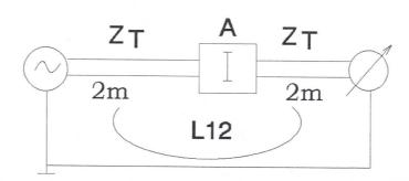
Guidance: To achieve  $\Delta = 0.1$  dB accuracy the "roundtrip" attenuation has to be about 40 dB above the attenuation of the test object. The attached monogram can be used.
