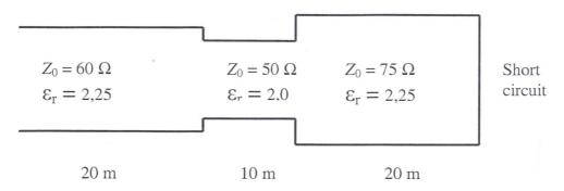
Draw the a) pulse response and b) step response and provide the figure with time and amplitude scale.
