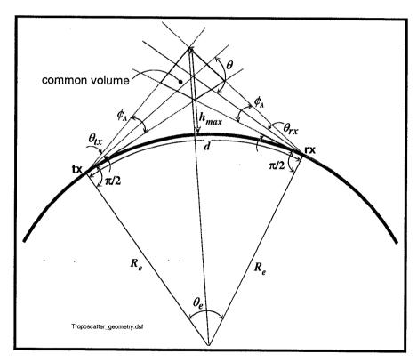
Based on the difference between the longest and shortest ray path in the tropo-scatter link geometry shown in the above figure, calculate the delay spread in the great circle plane assuming ideal conical antenna lobes just touching the ground as depicted in the figure. The path length along Earth's surface is 500 km,  $\phi_A = 1$  degree, and the equivalent Earth radius  $R_e$  is 8500 km. The propagation speed is assumed to be  $3 \cdot 10^8$  m/s.
