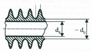
No exact value can be measured for the diameter du in the picture.
