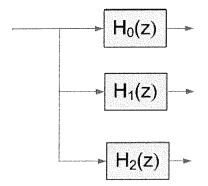
where  $h_i(n) = h(n)e^{j2\pi ni/3}$ . Determine the equivalent polyphase representation and draw its block diagram.
