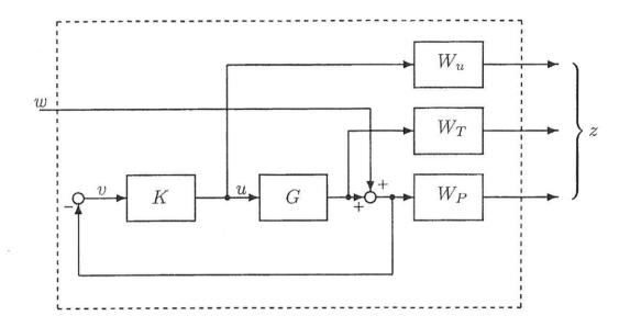
where G is the process, K the controller, Wu,  $W_T$  and  $W_P$  are weights.
