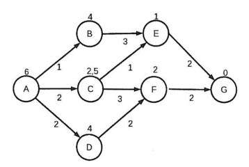
The aim is to find a path from state A to state G, when the values of function h are as shown in the figure on top of the states and the state transition costs are presented in connection to the arrows representing the transitions in the figure.
