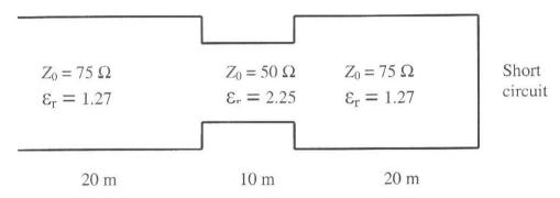
Draw the a) pulse response and b) step response and provide the figure with time and amplitude scale.
